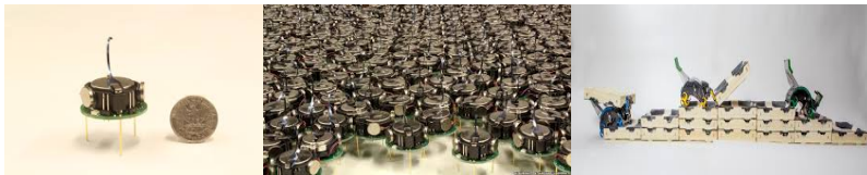
Figure: The Kilobot; A Kilobot swarm; Robots constructing a structure
